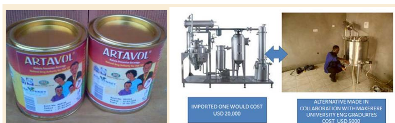
Fig. 7: Left: Artavol anti-malaria beverage. Right: Production equipment – extreme right is a locally fabricated version of the stainless steel equipment used for this pharmaceutical product.
